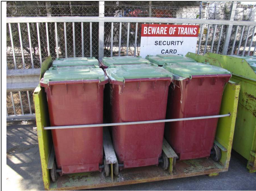
Purpose-built cradle for six 240 litre wheelie bins containing organic waste for disposal by EarthPower.
